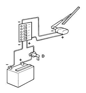
5. If an auxiliary battery is in use, a main switch (D) should be connected between its + terminal and the fuse block. The main switch for the auxiliary battery must cut off all power consuming equipment connected to that battery and be turned off when power is no longer needed.
