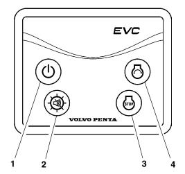
The system does not have an ignition switch. To stop unauthorized persons starting the engine the wheelhouse should have a lock or a lockable main switch should be used
